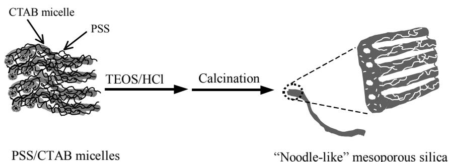
condensation of TEOS. The original PSS/CTAB templates were removed by calcination to yield mesopores. Finally, two kinds of mesopores were obtained from the contributions of CTAB micelles and PSS molecules, respectively.
