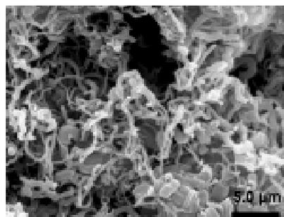
ratio plays a key role in the “noodle-like” particles’ structure formation. It was also found that the reaction temperature and ageing time did not make obvious differences in the silica morphologies. The adding sequence of PSS and CTAB also applied little
